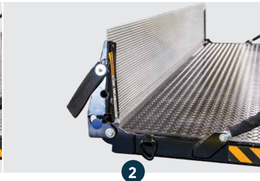
2 ramp locks at 90-degrees for cart retention
