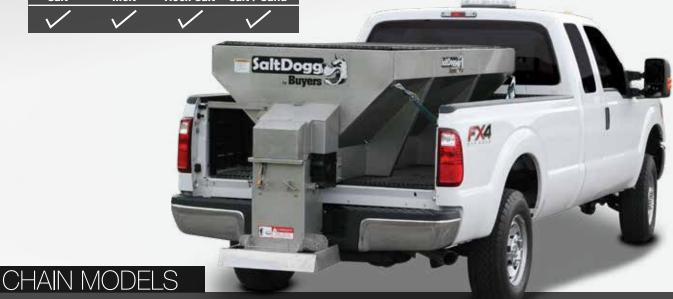
Feed Mechanism: 12 inch wide all steel pintle chain conveyor
