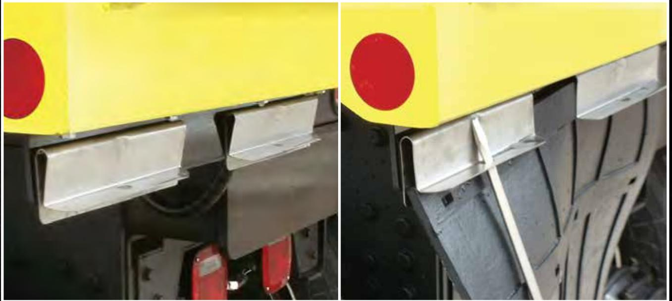
**DURABLE** - All stainless steel clamp construction, heat tempered to spring steel for ultimate durability.
