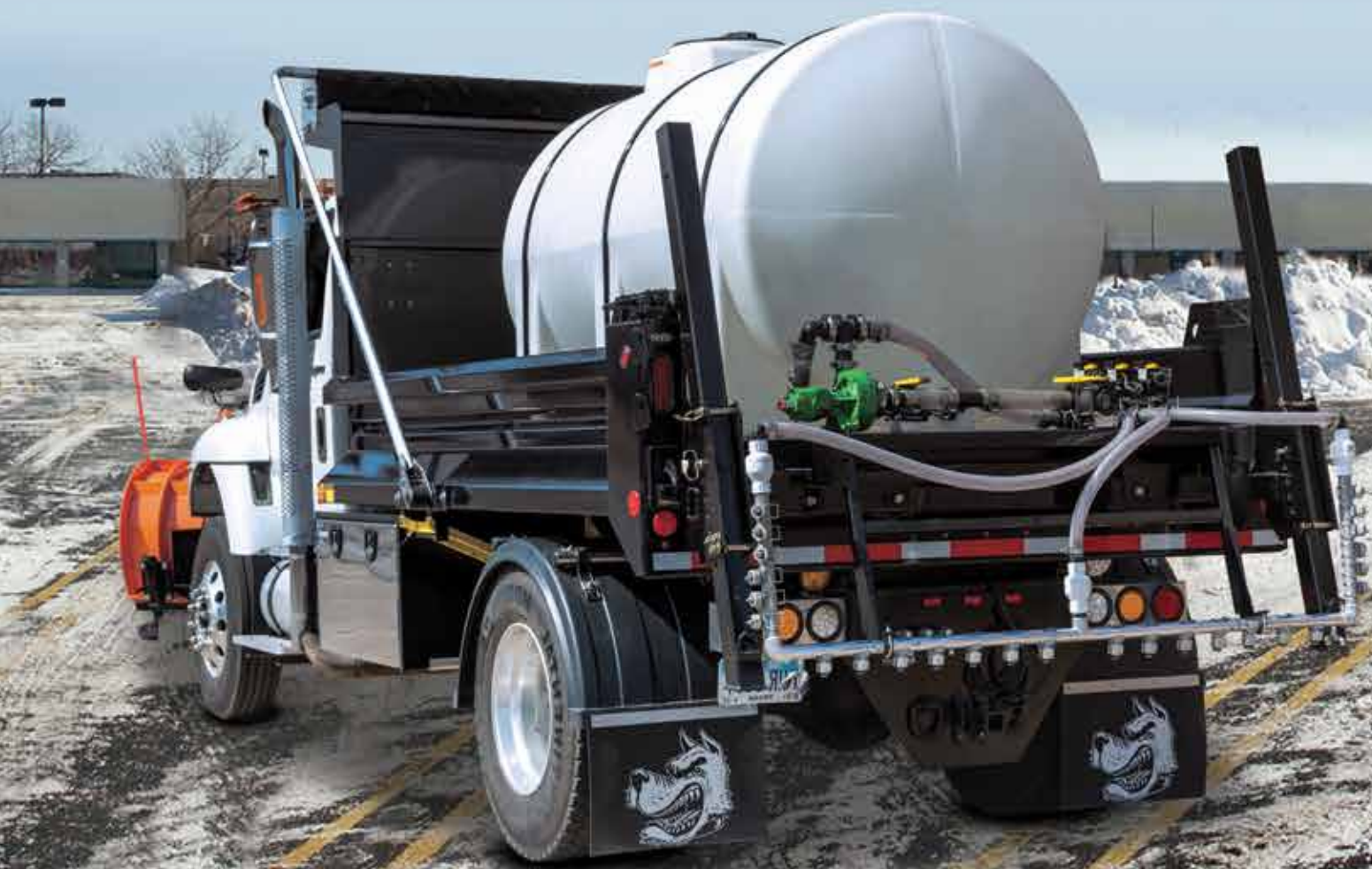
Hydraulic Systems - Powered by a 235 GPM hydraulic pump, with an oil requirement of 4-11 GPM
