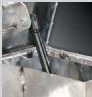
The cover support housing protects the gas springs
