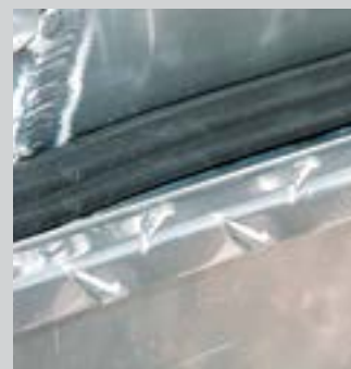
Full weather stripping keeps dust and moisture out
